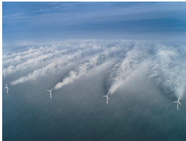
Figure 24: Photograph of Horns Rev 1 that depicts effects of leading turbines on trailing
