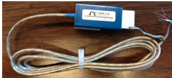
Figure 19: 5lbf load cell used in the force balance assembly.
