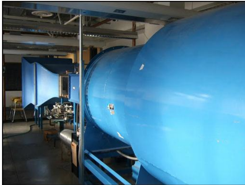
Figure 1: The ELD 404c Eiffel-type "Student Wind Tunnel" located in Kingsbury Hall, with test section dimensions W 18" x H 18" x L36",
