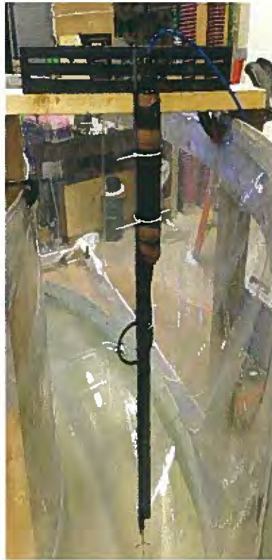
Figure 4-3: Vectrino II current profiler with mounting system.
