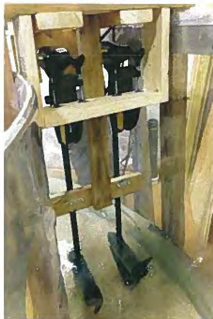
Figure 4-1: Dual 40 lb. thrust motors with mounting system.
