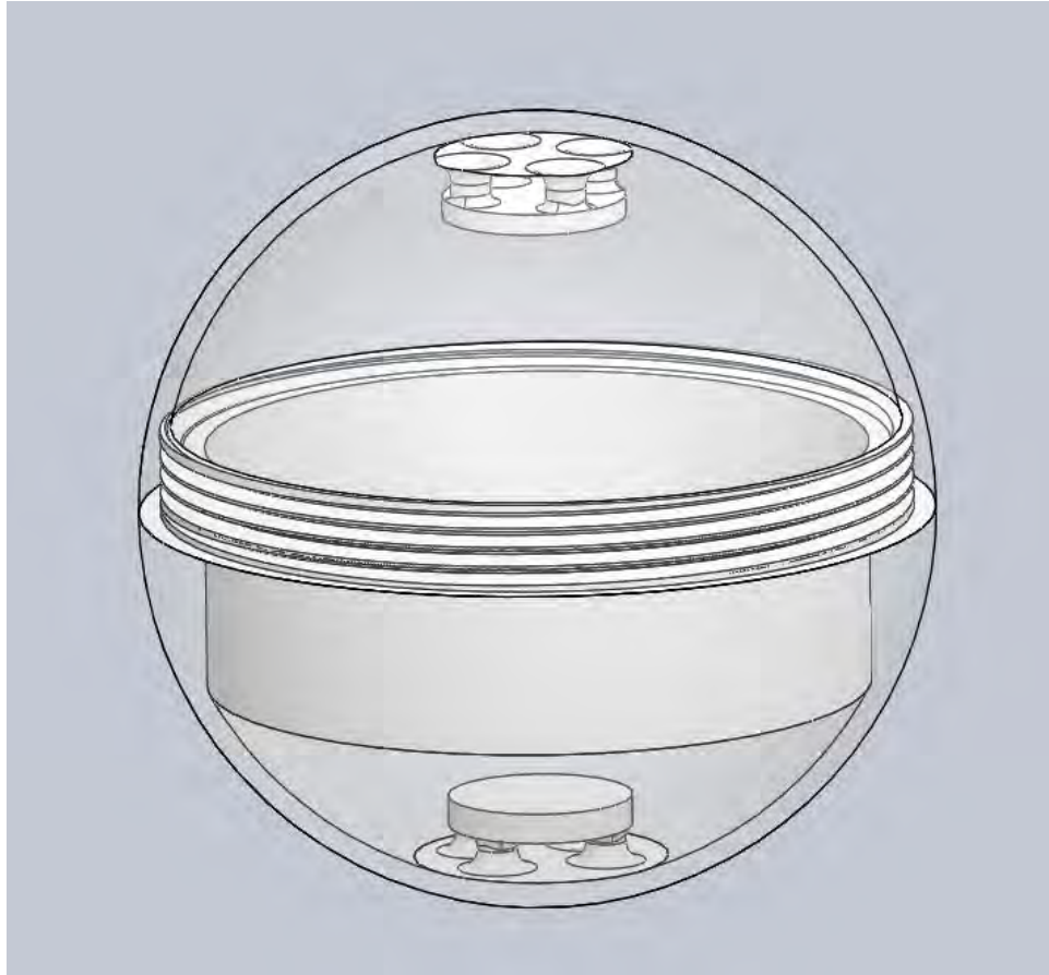
Figure 39: The two sphere halves assembled together. The transparency of the sphere was changed so the pedestals could be seen on each inner pole of the hemispheres. The solid wall just above the bottom pillar is the face that needed to be made in order to create the male threading. This wall could not be made transparent without the entire male half being made invisible.
