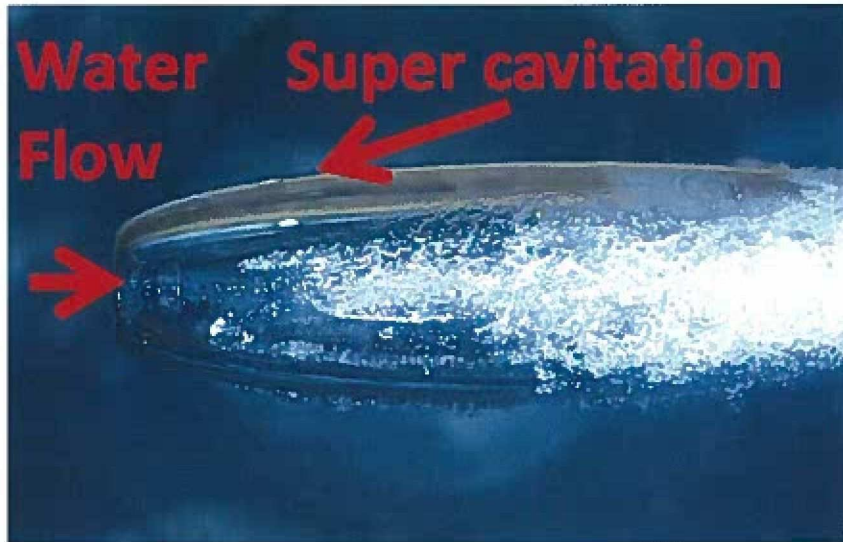
Figure 2: Example of an object travelling inside a supercavitation bubble (Wosnik et al. 2006)
