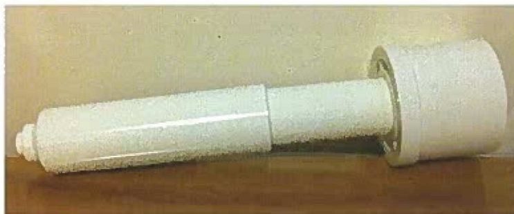
Figure 21: Simulated sensor made of toilet paper roll holder and PVC end cap
