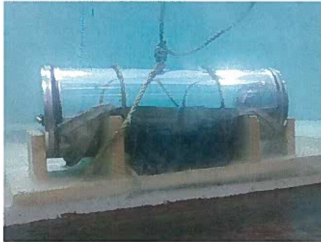
Figure 22: Electronics capsule attached to weights at bottom of Tow Tank in Jere A. Chase Ocean Engineering Laboratory
