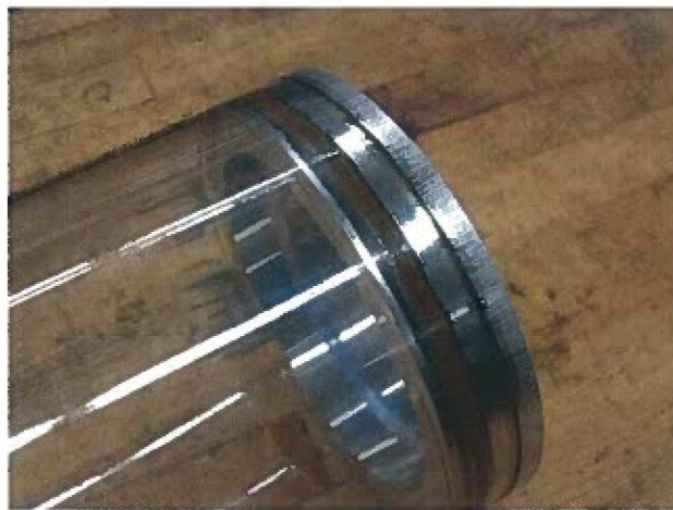
Figure 8: Electronics Capsule. An end cap for the electronics capsule is shown with O-Ring and polycarbonate cylinder.
