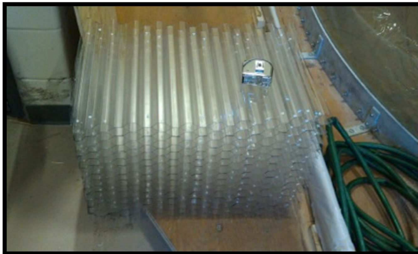
Figure 6: Final construction of the flow straightener
