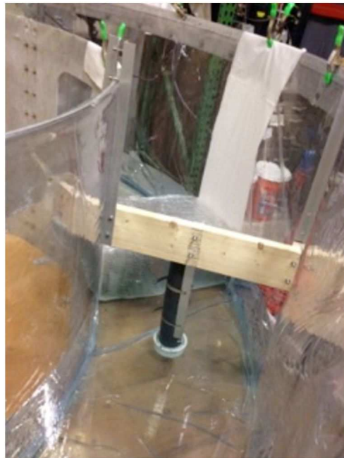
Figure 12: Camera pressure case, mount, and flow straightener
