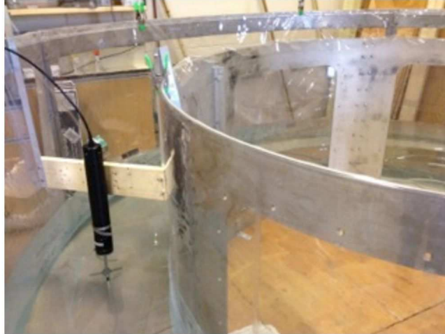
Figure 9: Vector being used to collect velocity measurements in the tank
