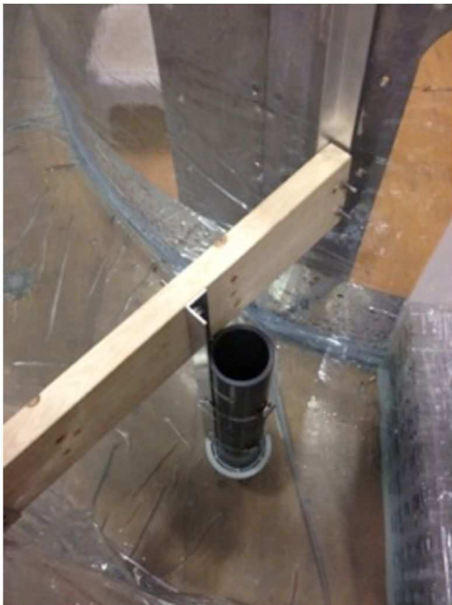
Figure 11: Camera pressure case and mount
