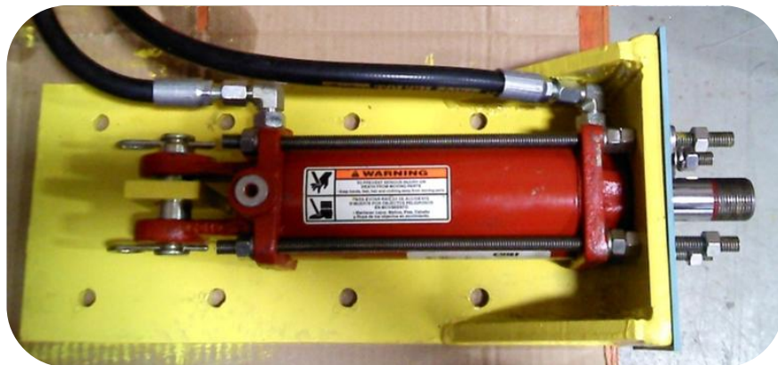
Figure 5.4: Hydraulic cylinder pictured with mounting bracket
