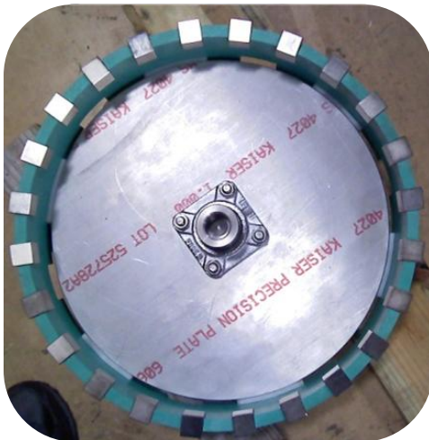
Figure 6.5: Aluminum rotor hub with magnet ring attached
