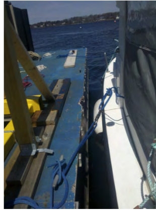
Figure 32: Hip Tow setup with Galen J. boat and Force Transducer
