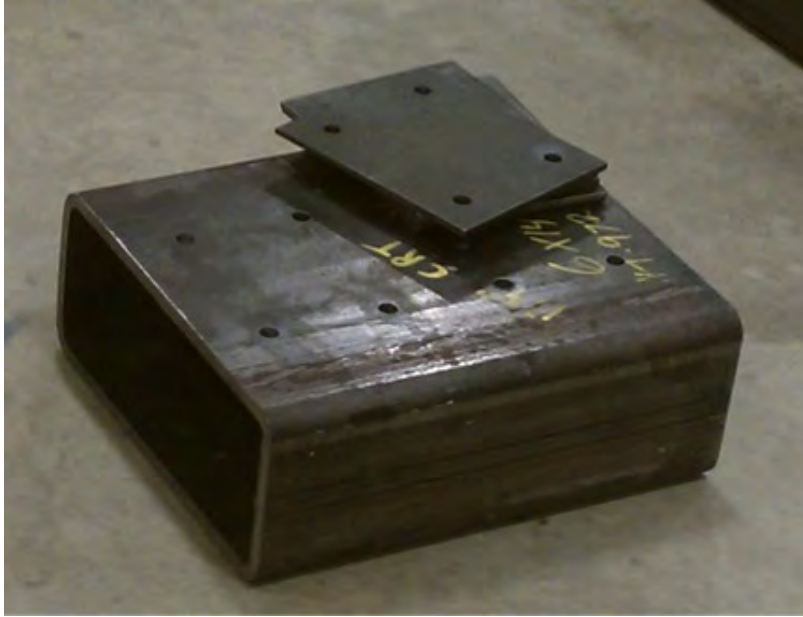
Figure 29: Completed box assembly
