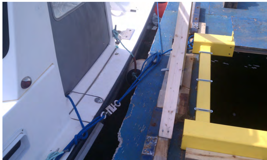
Figure 24: Hip-Towing the barge using the Galen J
