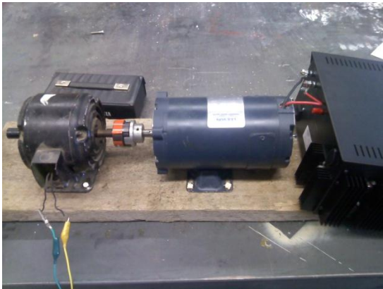
Figure 10: Experimental Set-up for motor time response. Photo on the left is a portion of the actual set-up for the system, and the diagram of the right shows a pictorial representation of the experimental set-up.
