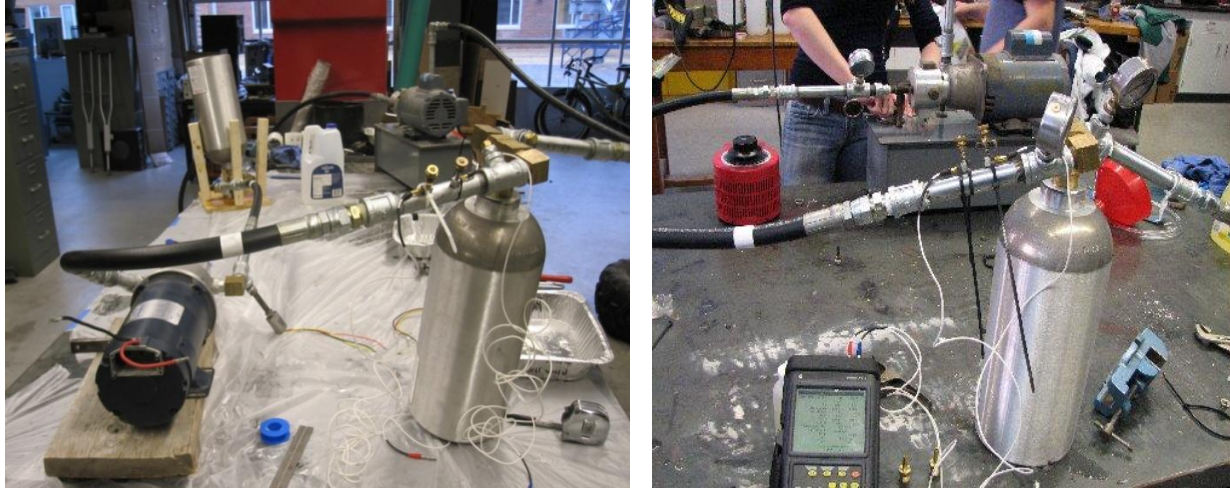
Figure 14: Hydraulic system, benchmark testing area. The photo on the left shows the entire hydraulic system with the pressure transducer attached in front of the generator. The photo on the right shows the flow meter used to take the volumetric flow rate during the testing.
