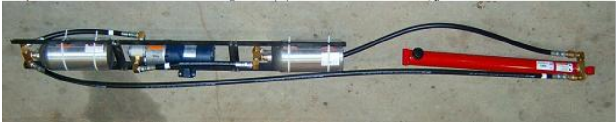
Figure 8: Hydraulic system set-up for testing done on the accumulator. This photo was provided by the 2008-2009 Wave Energy Conservation group.
