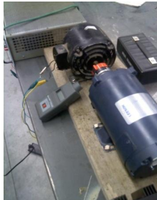
Figure 11: Experimental set-up for motor time constant, showing where the tachometer sits to read the shaft speed.
