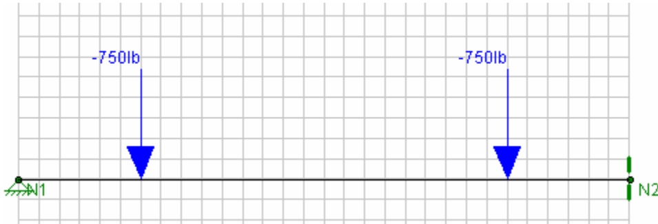
Figure 34: Deck Beam Loading for Cage Short (RISA)
