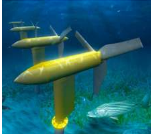
Figure 9: Propeller Style Tidal Turbines.
