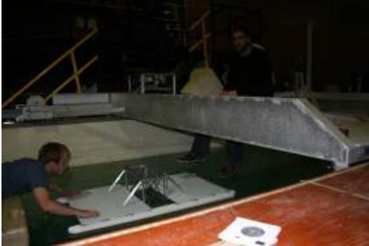
Figure 25: Installing the Tow Bridal
