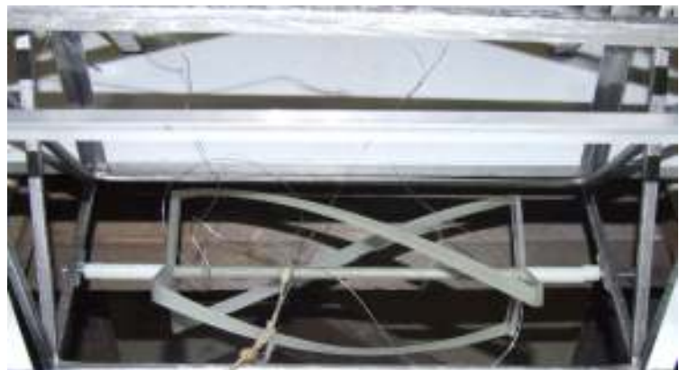
Figure 28: Gorlov Test Turbine
