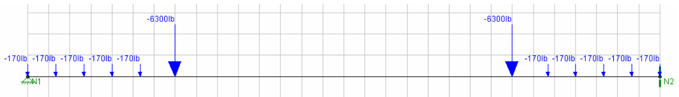
Figure 43: Transverse Derrick Support Beam Worst Case Loading
