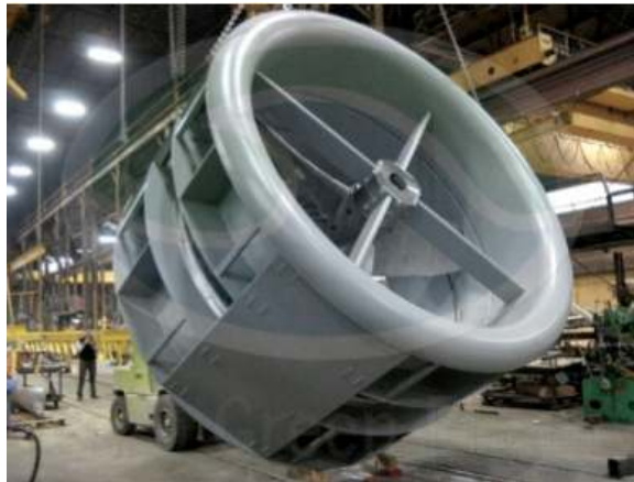
Figure 10: Ducted Style Hydrokinetic Turbine.
