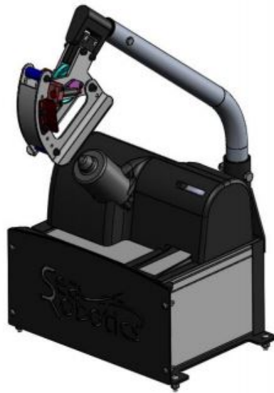
Figure 4: SeaRobotics lightweight wire line winch
