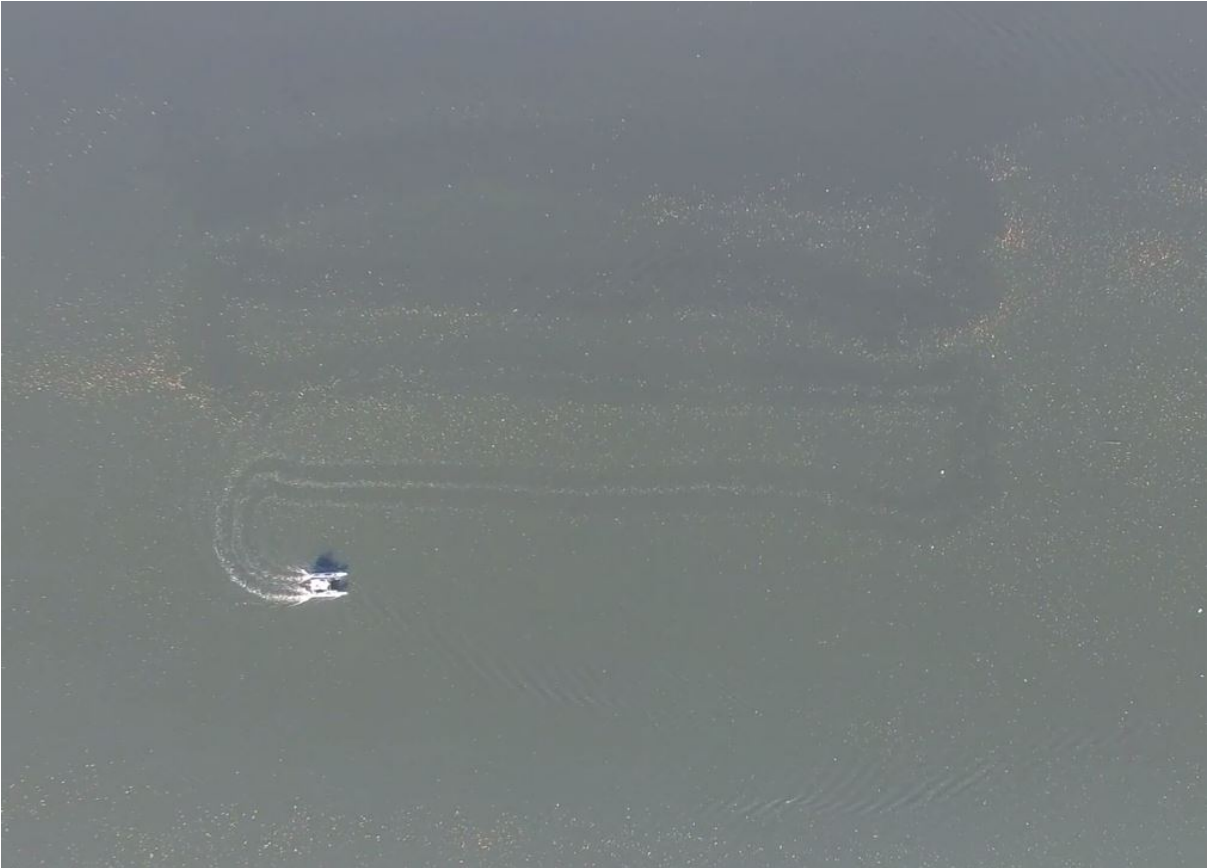
Figure 26: REx 4 performing a “lawnmower” search pattern on the Charles River
