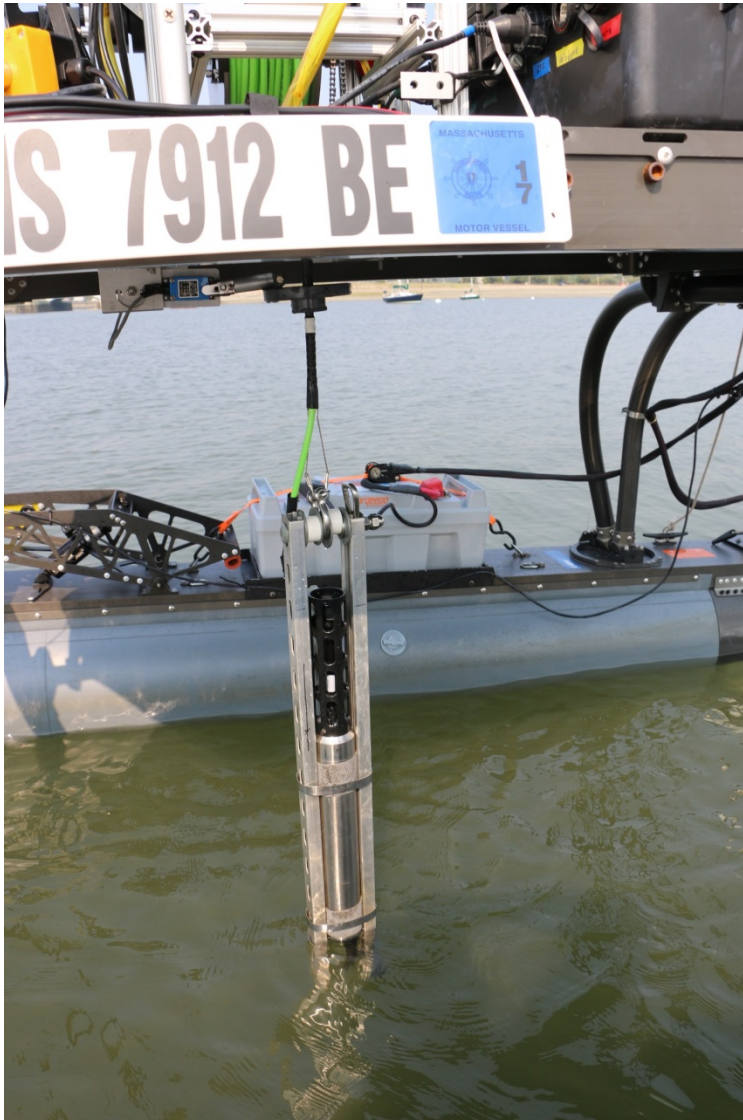
Figure 8: CTD sensor and tether detail
