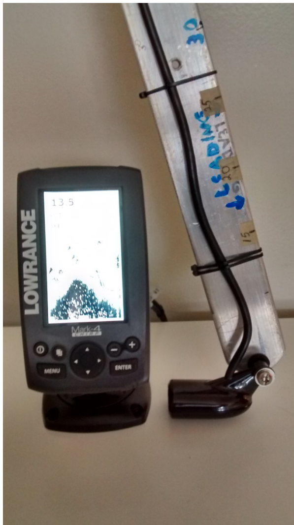
Figure 9: Lowrance Mark 4 sonar and mounting arm
