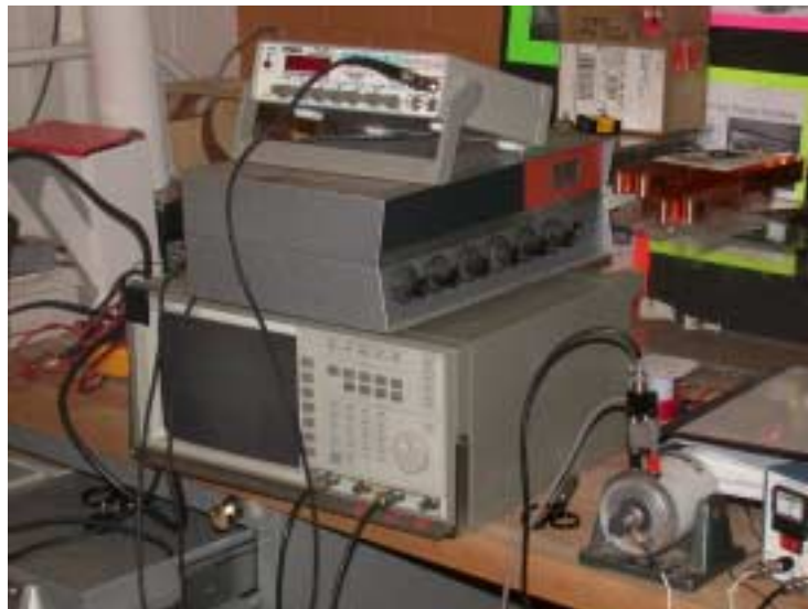
Figure 7.11 - Photograph showing mass shaker used on top of cassette for response measurements
