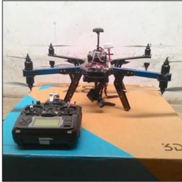
Figure 4 : X8+ Octocopter manufactured by 3DR
