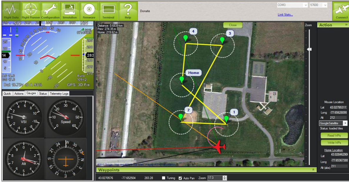
Figure 8: Flight path of a drone during a mission (source: google images)
