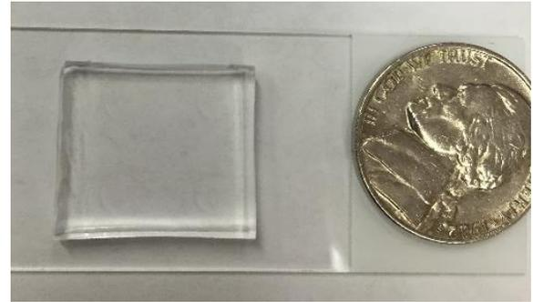
Figure 6. Base component of the microfabricated enumeration grid chamber (MEGC)
