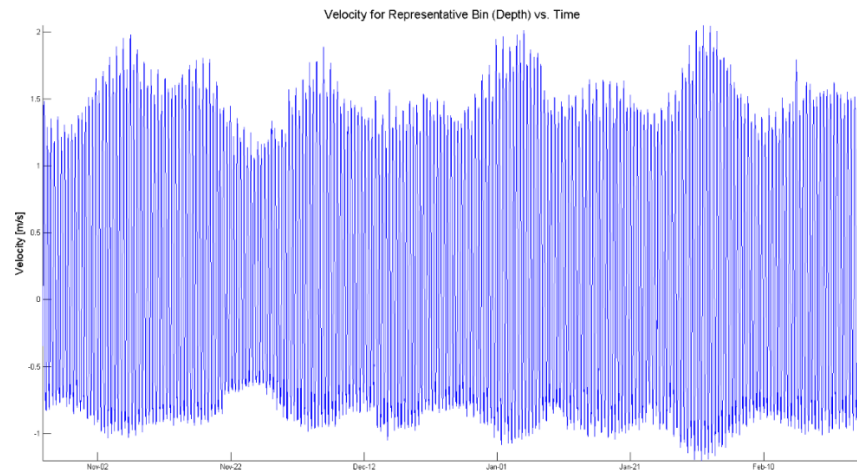
Figure 29: Tidal current velocity for representative depth versus time that the measurement was recorded
