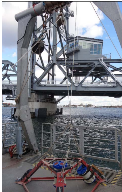
Figure 3: Equipment utilized for the acquisition of tidal current velocity measurements for performing a detailed tidal energy resource assessment
