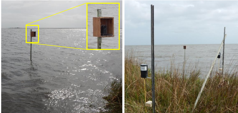
Fig. 8. Time-lapse camera after installation
