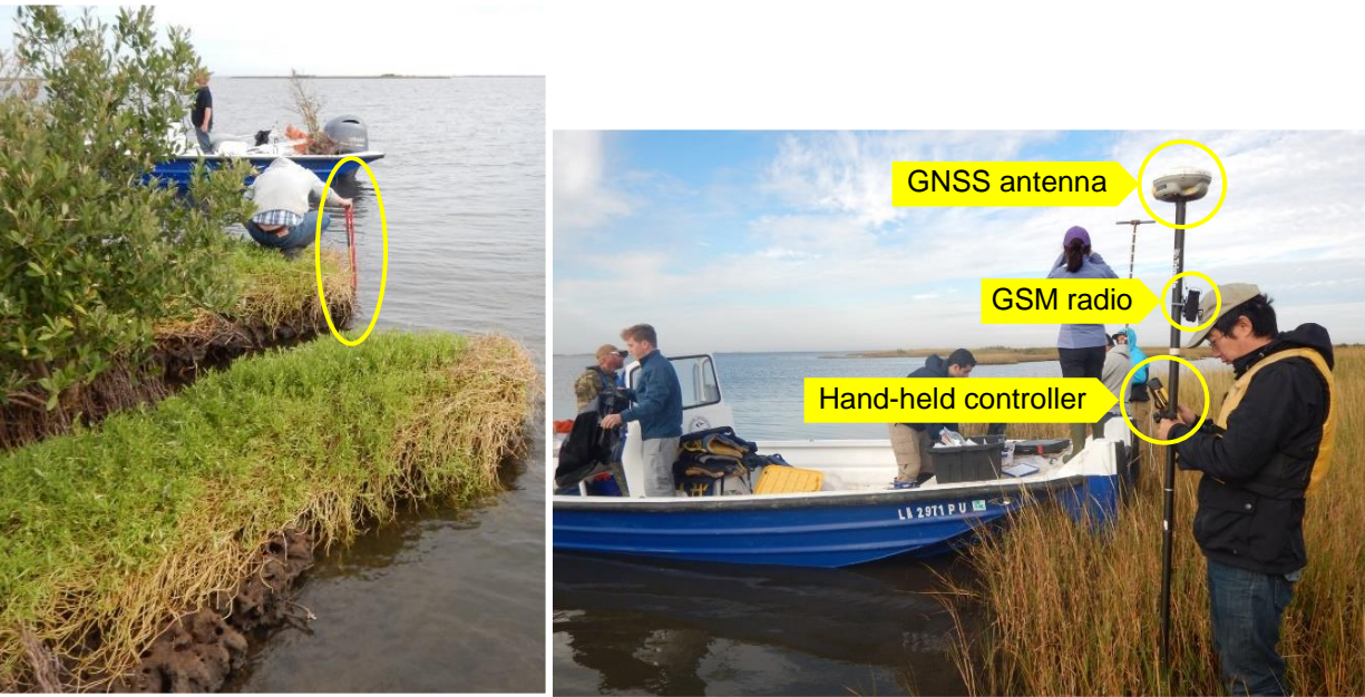
Fig. 6. Measuring scarp height using a metric ruler (left) and RTK unit (right)
