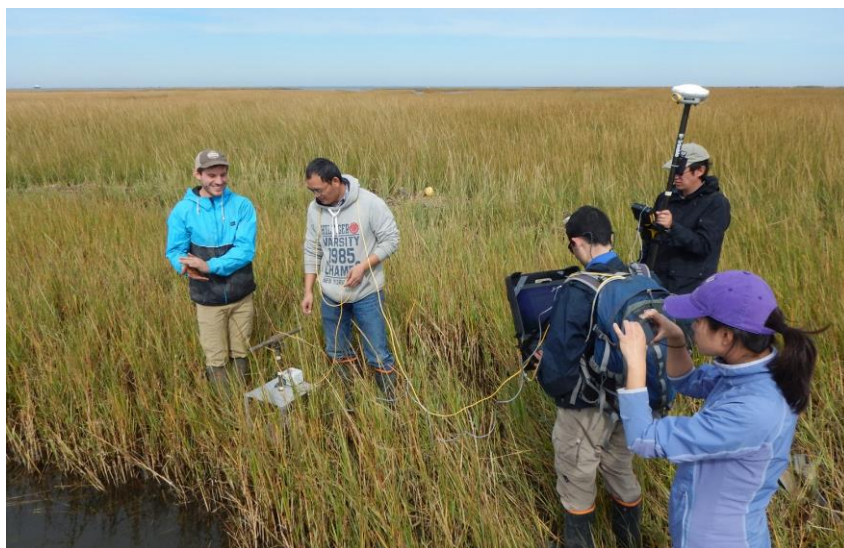
Fig. 7. Configuring the RTK unit to record location of a recently completed cone penetration test
