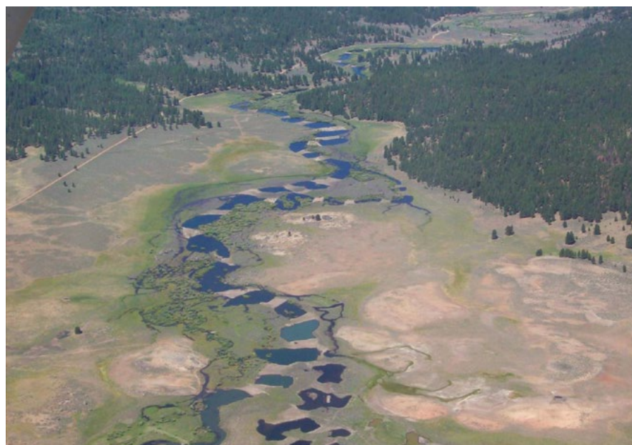
Image 3: Pond-and-plug floodplain restoration on McReynolds Creek in the Sierra Nevada mountains in California (from Wilcox 2010)
