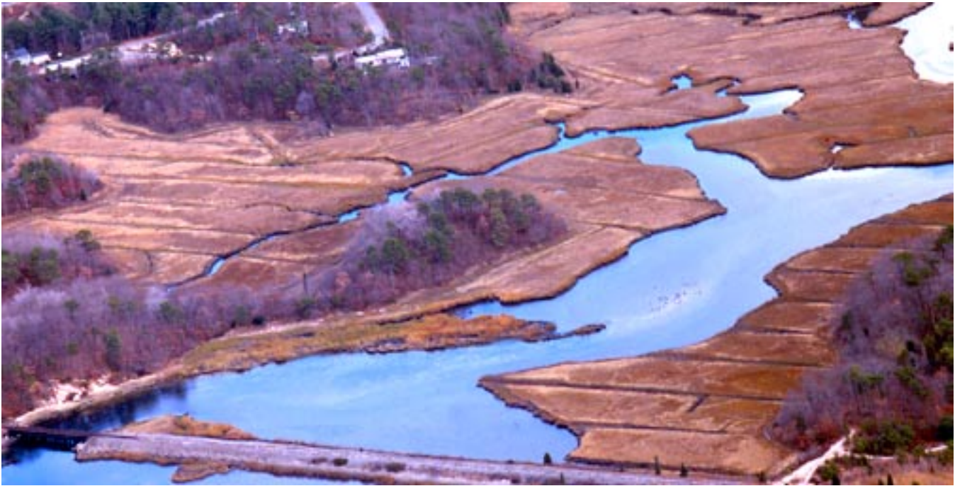
Road crossings and human-made ditches (visible as straight lines) intended for mosquito control and draining harm the health of many salt marshes around the Gulf of Maine. Massachusetts ACEC Program
