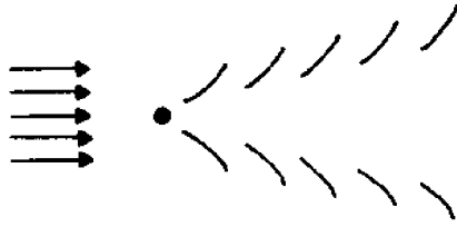
Fig. 6. Schematic illustration of a wake caused by an obstacle in a uniform flow in a fluid with a free surface. Such wakes are apparent in patterns of low, stratiform clouds downstream of small islands.
