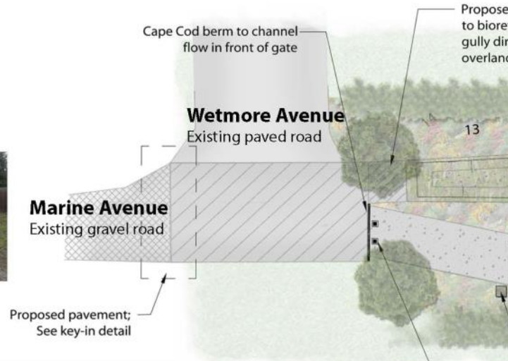
The stormwater runoff from the watershed (275,000 sqft, 6.3 acres) is captured in the proposed bioretention basin, see Appendix X for sizing information
