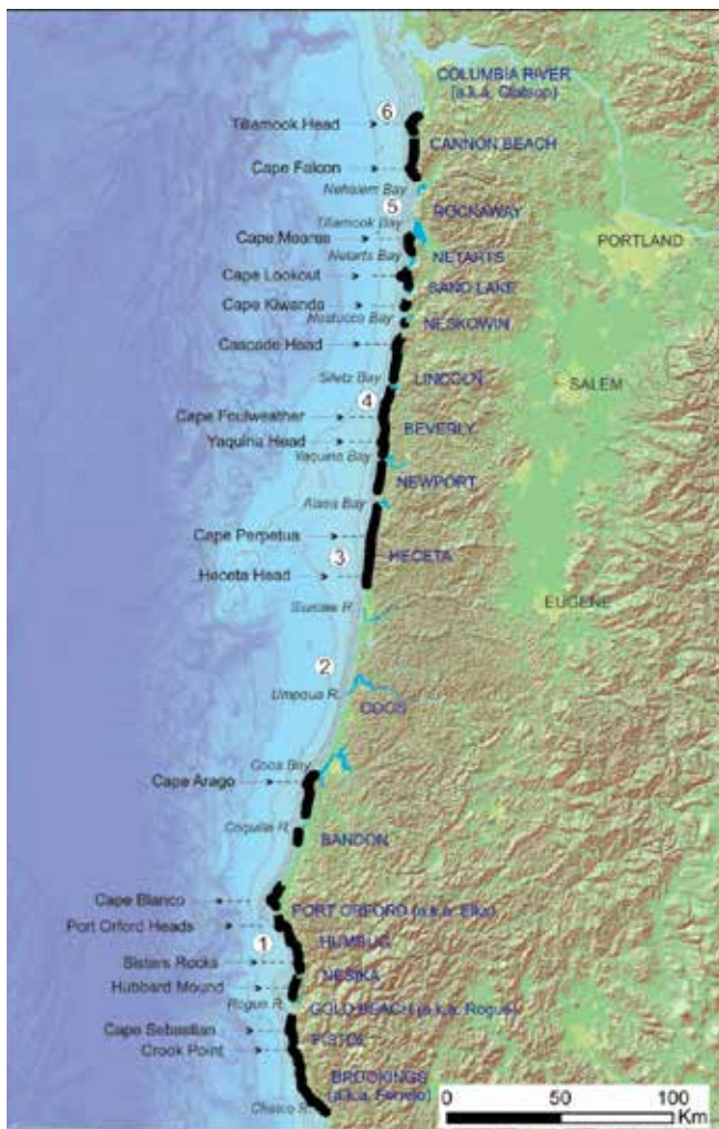
Figure 1. The coastal geomorphology of the Oregon coast, including a breakdown of Oregon littoral cells. Bold black lines denote the locations of cliffs and rocky shores. Numbers indicate regional coastal geomorphic features: plunging cliffs (1, 4 & 5), rocky shorelines and shore platforms (1, 3, 5 & 6), wide and narrow sandy beaches backed by both dunes (2, 5 & 6) and cliffs (3 & 4), gravel and cobble beaches backed by cliffs (1, 5 & 6), barrier spits (2 & 5), and estuaries (1-6).
