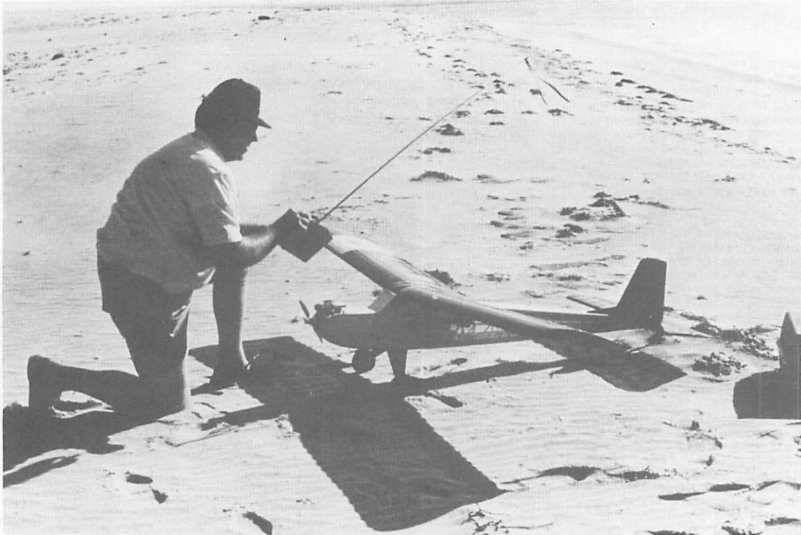
Figure 3. Fritz Hess developed the radio-controlled model airplane shown in the figure for Lagrangian flow measurements in a tidal inlet environment. (David Aubrey)
