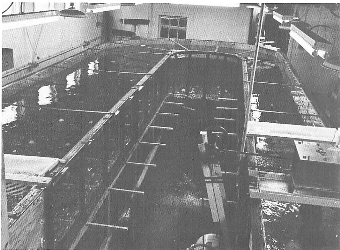
Oblique view of experimental stream tank, with 4 ft. wide channel on left, 2 ft. wide channel on right and 5 ft. wide pool at top.
