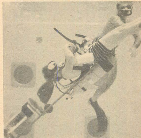
Scuba divers test Seireg's underwater diver orientation device.
