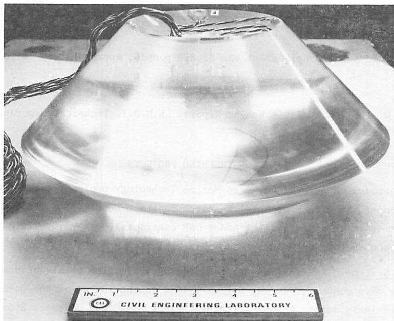
Fig.3 (Shumaker) Spherical Sector Window showing Strain Gauge Attachments.
