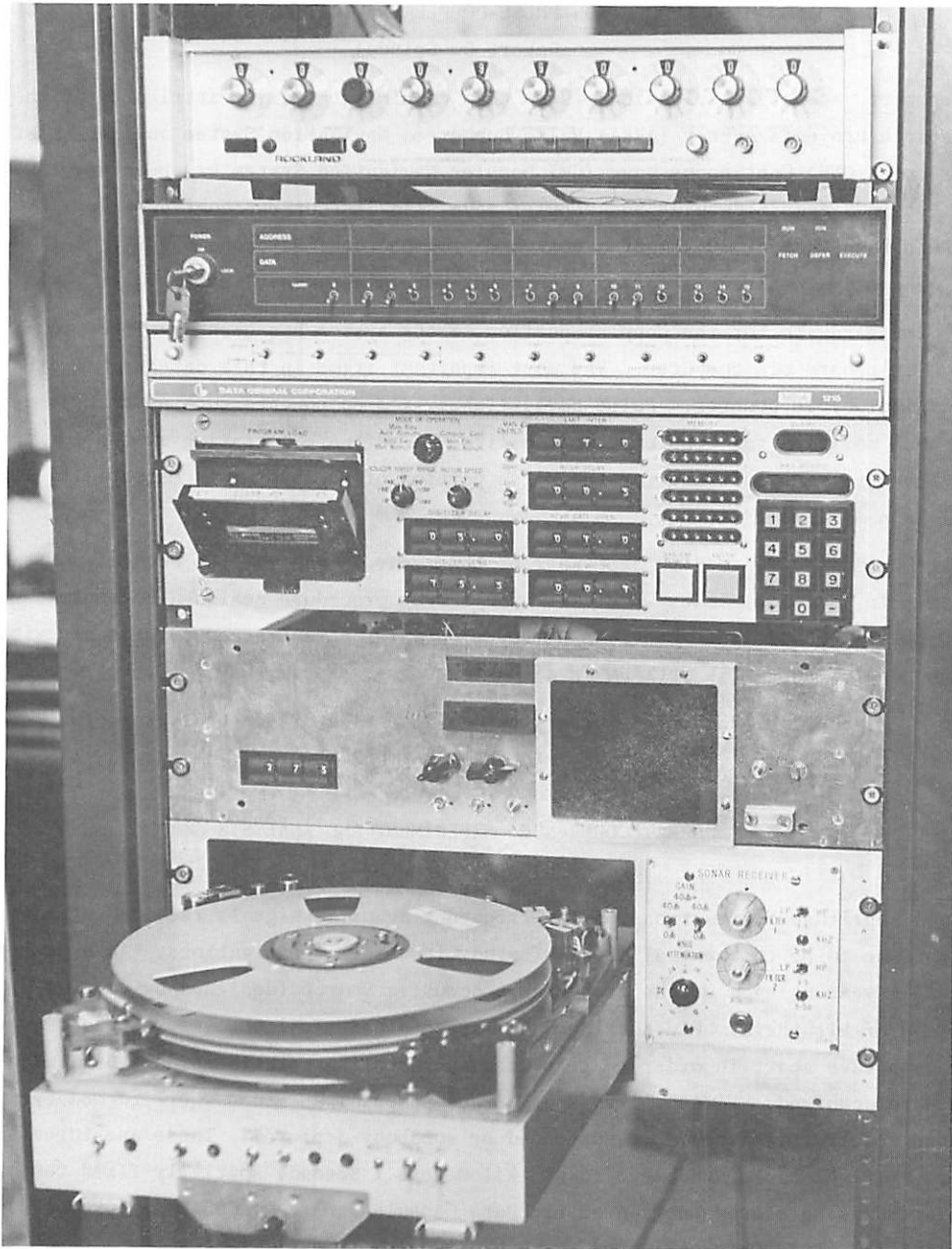
Fig.1 (McElroy and Hess). Inboard components of the submersible system arranged from top to bottom as follows: Rockland frequency synthesizer; Nova 1210 computer; control unit containing Ross cassette, manual control thumbwheels, and keyboard with echo display; display unit with transducer-pedestal azimuth and elevation readouts; tunable receiver, and the data/logging tape recorder.
