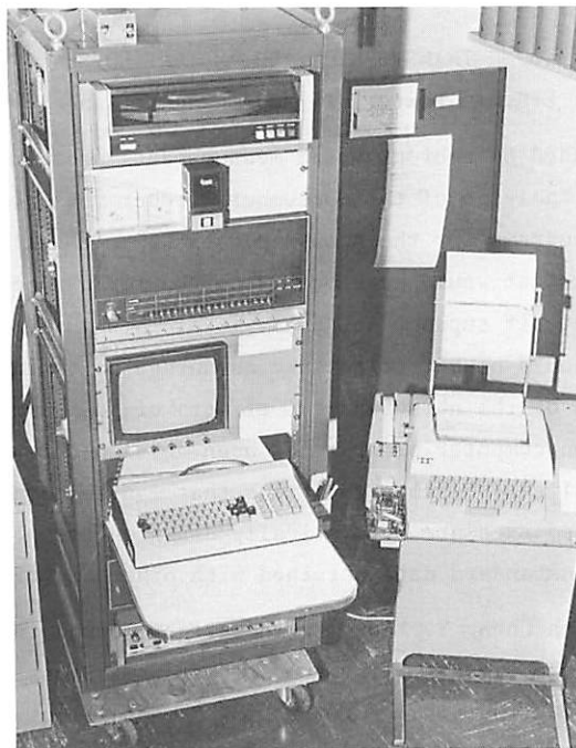
Fig.3 (McElroy and Hess) Surface computer system. Repco high speed printer at left rack, Top to Bottom: Disc Storage Unit, Remex High Speed Tape Reader NOVA 1220 CPU, Scope Graphics Terminal, Keyboard, Disc Controller (under table). ASR-33 Teletype at Right.
