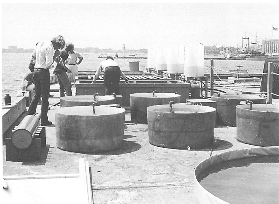
Fig. B-3 (Ryther) Output of the algal culture tanks are pumped into the white, polyethylene food reservoirs in the background. From there algae, together with filtered seawater, are fed into the rectangular (500 gal) animal tanks.
