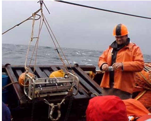
Figure 1. Drop camera system used in the Aleutian Islands in the summer of 2003.
