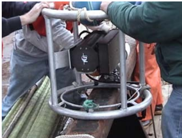
Figure 1. A DIDSON acoustic camera within its protective housing.
