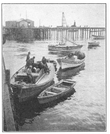
FIG. 7. Flat-bottomed lighter, skiff and launch with lampara piled in the stern. The second launch (center background) is a salmon troller with short mast and outrigger "poles." Photograph by W. L. Scofield, Monterey, July, 1919.
