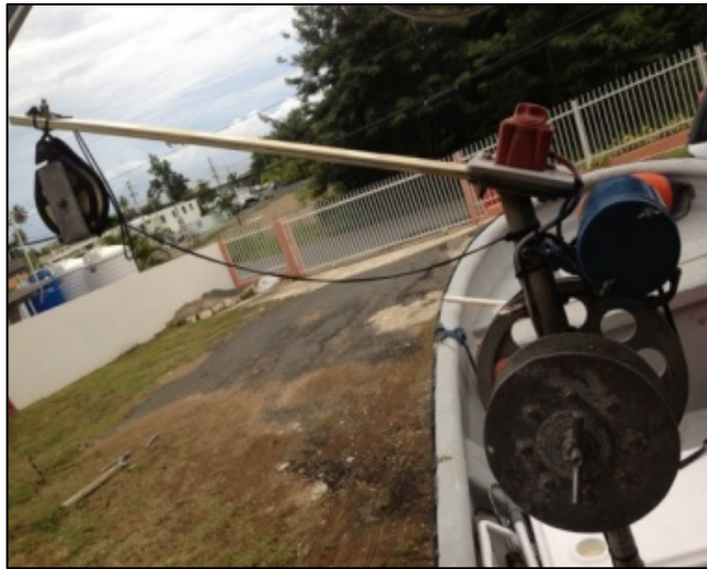
Automatic reel used for deep-water snapper fishing in Puerto Rico. (Source: E. Piñeiro)
