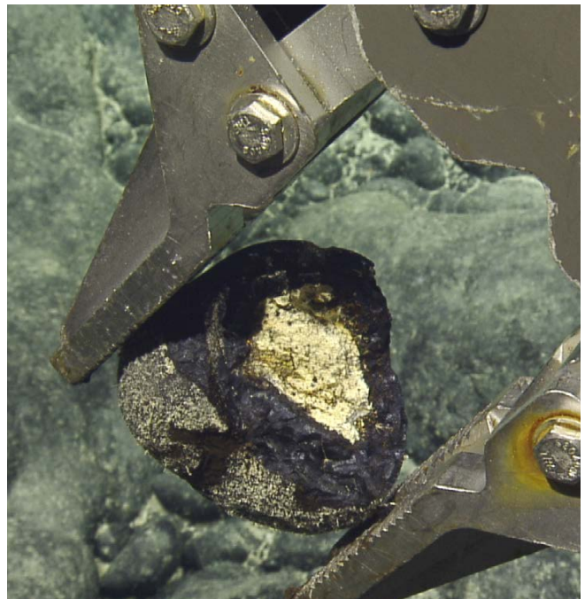
FIGURE 2. The arm of ROV Hercules collects an altered rock sample for analysis of microbial ecosystem services and mineral content in seamount rocks.
