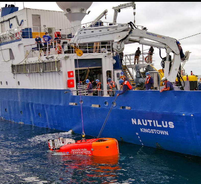
FIGURE 1. Launching Woods Hole Oceanographic Institution's hybrid remotely operated vehicle Nereid Under Ice (NUI) from E/V Nautilus . Photo credit: OET
