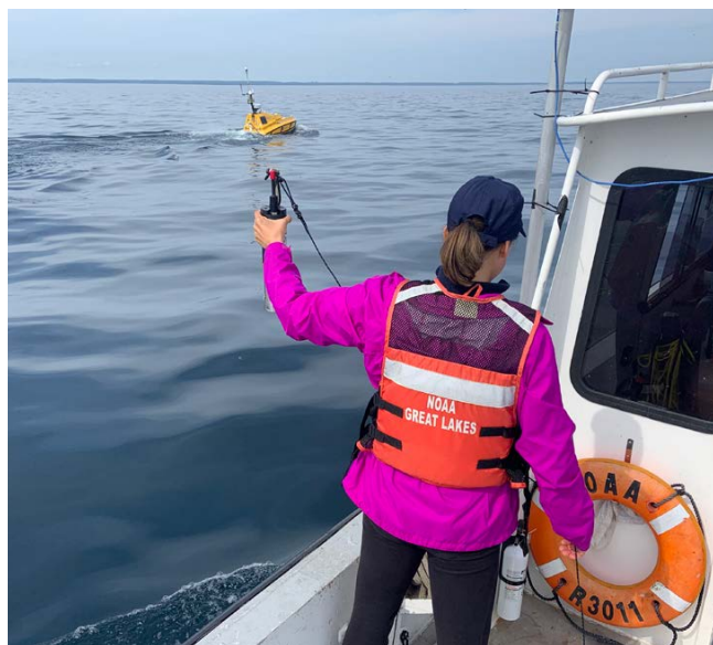
FIGURE 2. NOAA R/V 3011 tracks autonomous surface vehicle (ASV) BEN during mapping operations. Once in range, sound velocity cast data are wirelessly transmitted to BEN .
