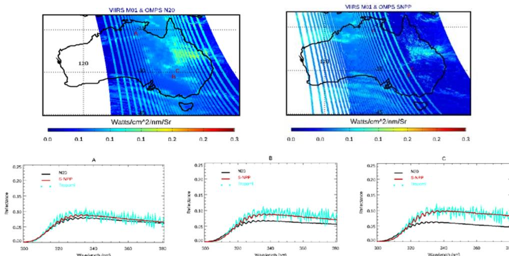
Figure 2 VIIRS Channel 1 on NOAA-20 overlaid with OMPS on NOAA-20 (upper left) and OMPS on S-NPP (upper right). Lower three panels are spectral in the three pixels A, B and C as marked in upper panels.
