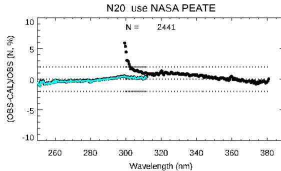
Figure 5 Comparison of OMPS N20 spectral with the simulations using inputs from NASA S-NPP EDR data. Orange line is for NP channels and black dots is for NM channels.
