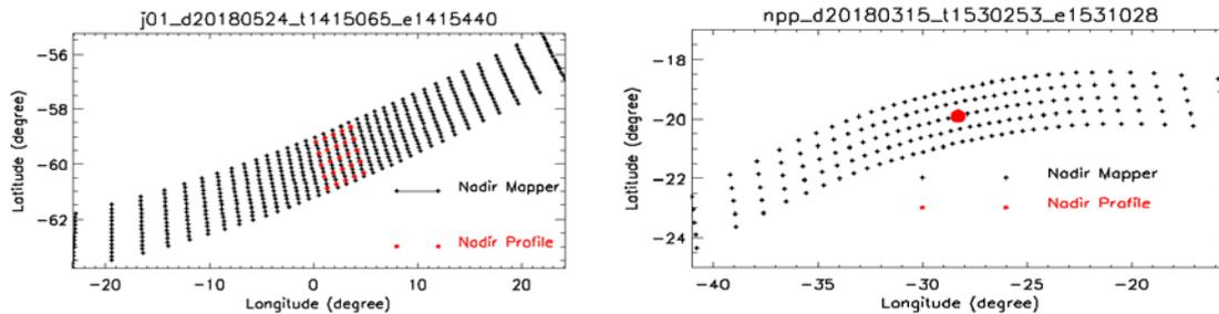
Figure 1 Sampling patterns of NM & NP for OMPS on N20 (left) and its comparison with OMPS on S-NPP (right). Red dots are for N20 and black dots are for S-NPP for one granule.
