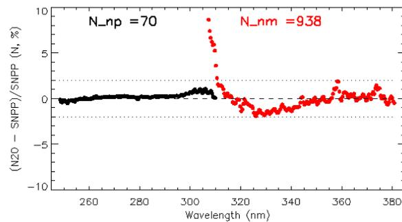
Figure 3 Comparison of N20 spectral with S-NPP spectral. Black dots are for NP channels, and red dots are for NM channels.
