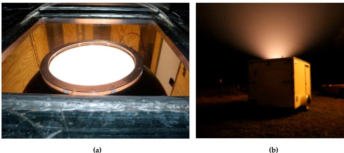
Figure 7. Terra Vega installed within a trailer (a) beneath a protected window with retractable cover and (b) in operation at the South Dakota site.
