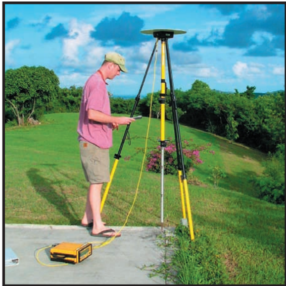
Figure 2.2. Taking GPS data to orthorectify aerial photographs.
