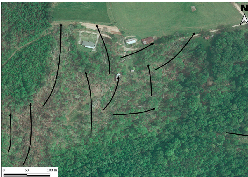
FIG. 7. Aerial imagery highlighting the likely transition between tornado damage (south–north tree falls on the left) and RFD microburst damage (west–east tree falls on the right) near the area of maximum continuous damage width.
