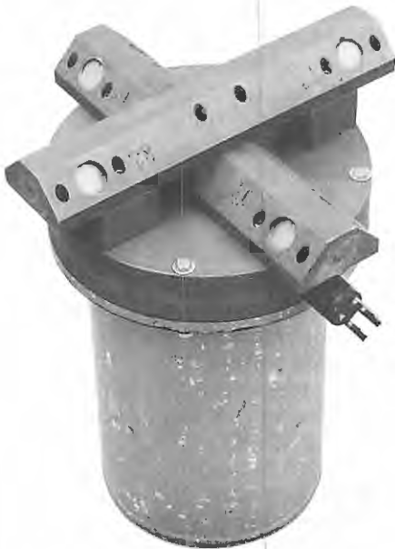
Figure 1. Continuous-wave Doppler acoustic instrument. The instrument case is 30 cm tall and 20 cm in diameter.
