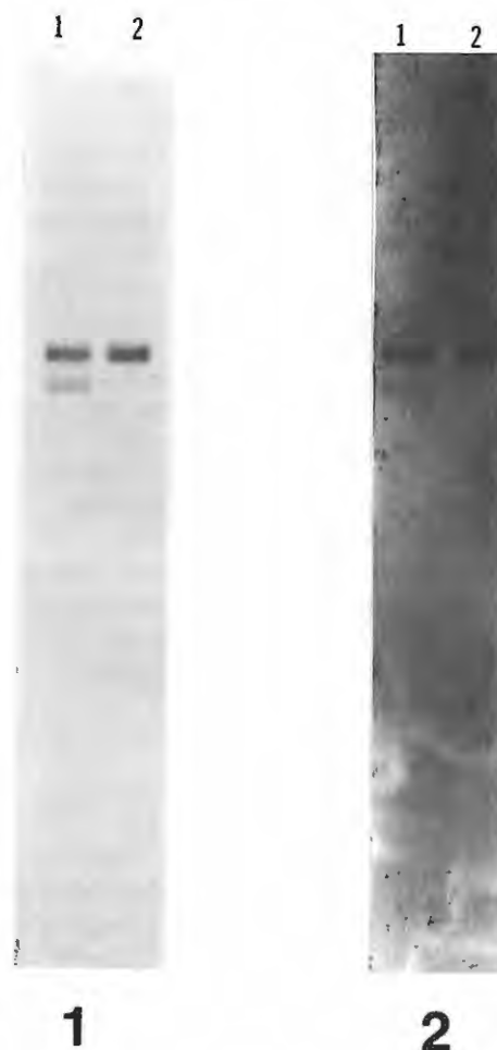
Figure 1. Southern blot of Anisakis DNA hybridized with the nonradioactively labeled Anisakis probe. Southern blot 1 was probed with radioactively labeled ( ^{32}\text{P} -dCTP) probe. Southern blot 2 was probed with nonradioactively labeled probe. Lane 1, Anisakis DNA cut with EcoRI and Lane 2, Anisakis DNA cut with Hind III.
