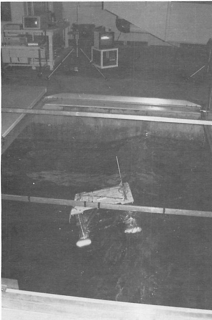
Figure 1. Experimental setup of Ocean Ranger model in listed configuration subject to large-amplitude planar wave.
