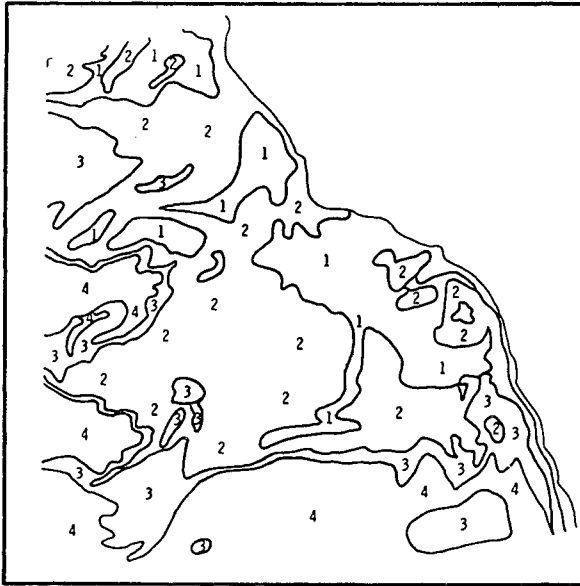
Figure 7. A color boundary chart constructed from a false-color enhanced CZCS image. Key water masses are identified by numbers. Geographic landmarks are added to chart before transmission by radio-facsimile.
