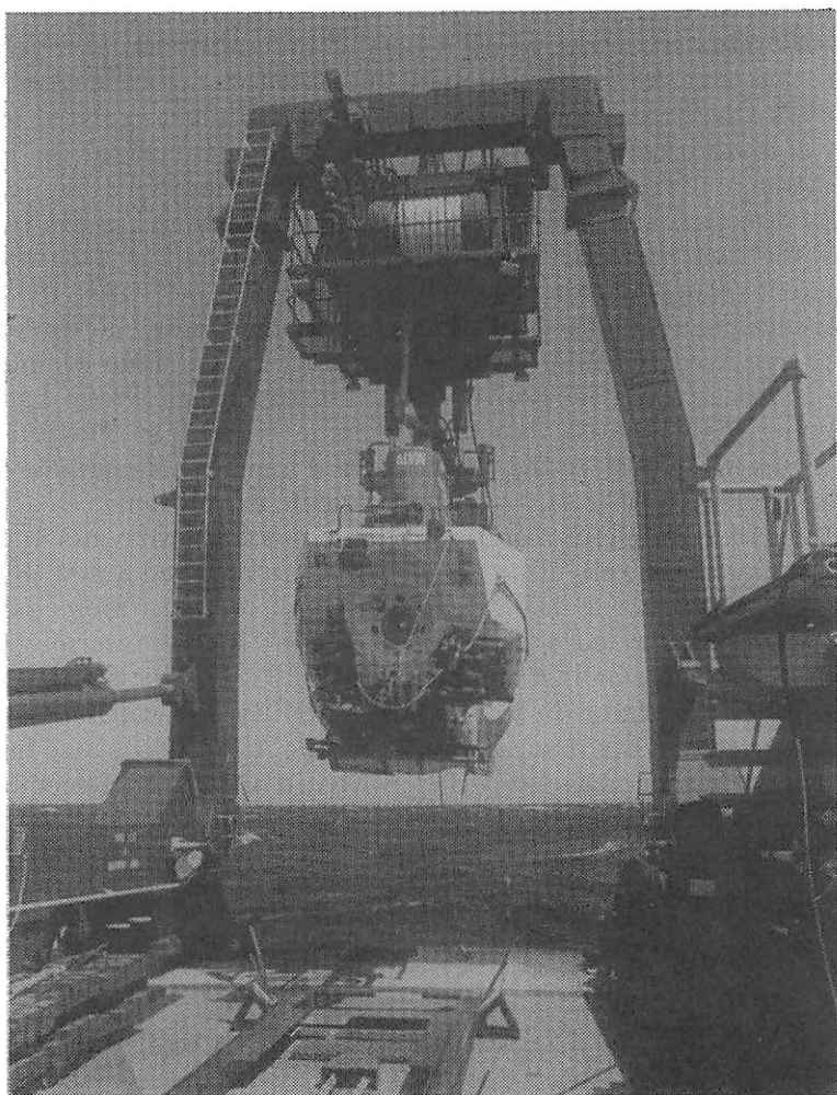
Fig. 2. Recovery of DSV Alvin aboard its support ship Atlantis II.
