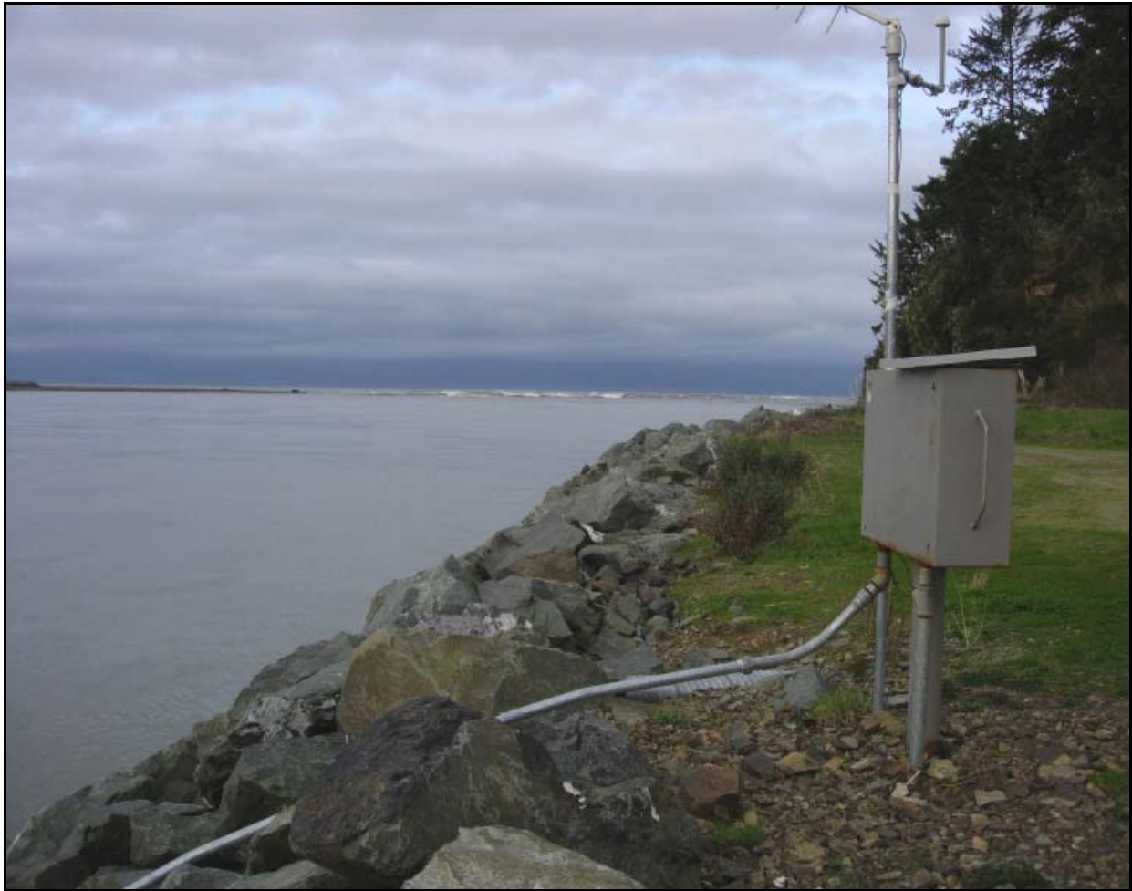
Figure 14. LES gaging station location at the downstream end of the RV park and campground. Note ocean waves in the distance.
