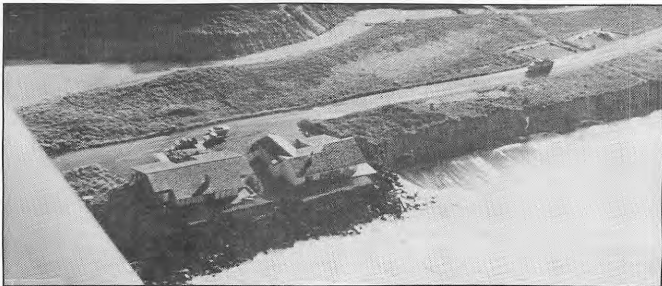
Paul Komar's research showed that property damage at Siletz Spit in 1972 could have been prevented with more adequate setbacks.
