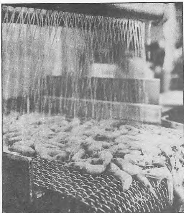
Application of phosphates before pre-cooking raises the commercial yield of cooked shrimp meat by approximately 33 percent.
