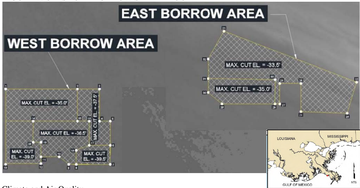
FIGURE 5. OFFSHORE BORROW SITE LAYOUT
