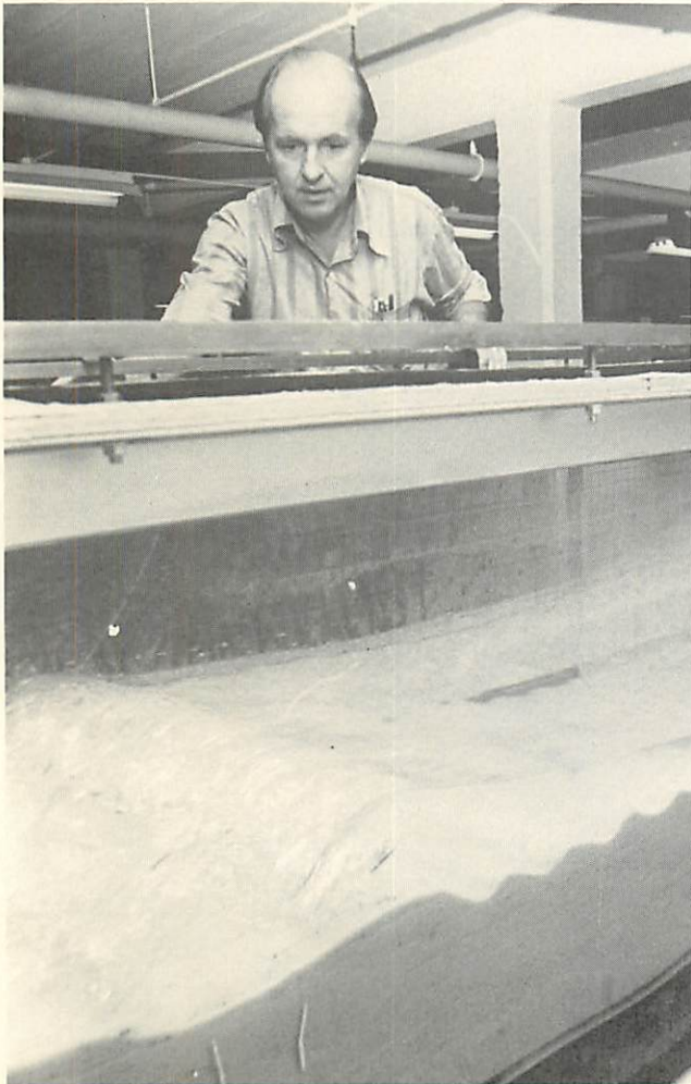
Dr. John Herbich of A&M's Civil Engineering Program uses a wave tank model to study scour around pipelines such as those used in the offshore industry. Photo by Austin Stockton.
