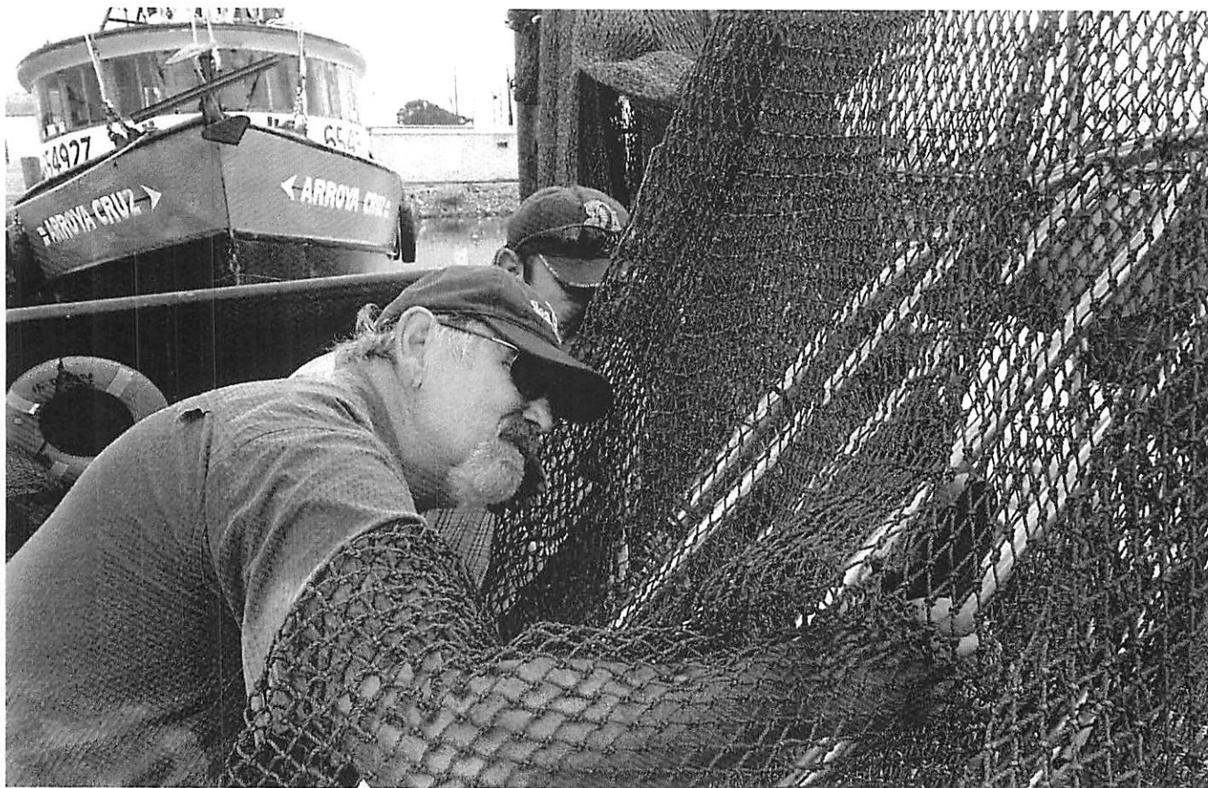
Texas Sea Grant College Program Fisheries Specialist Gary Graham (foreground) measures the angle of a turtle excluder device in a shrimp net aboard a boat in Brownsville to confirm it complies with federal regulations. Photo by Tony Reisinger, courtesy Texas Sea Grant.
