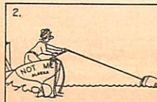
2. WITHDRAW ALL THE PAINTER TO INFLATE RAFT.
