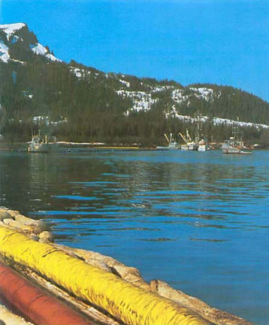
Left—Oil containment booms protecting a Prince William Sound salmon hatchery. Booms work like floating fences. Some block the spread of oil slicks, others also absorb oil. Different booms are used in open ocean, protected waters, and icy conditions. Below—Containment boom towed by two fishing vessels funnels oil slick into a weir skimmer. Lower left—Residents of Homer, Alaska, built booms by strapping logs together.
