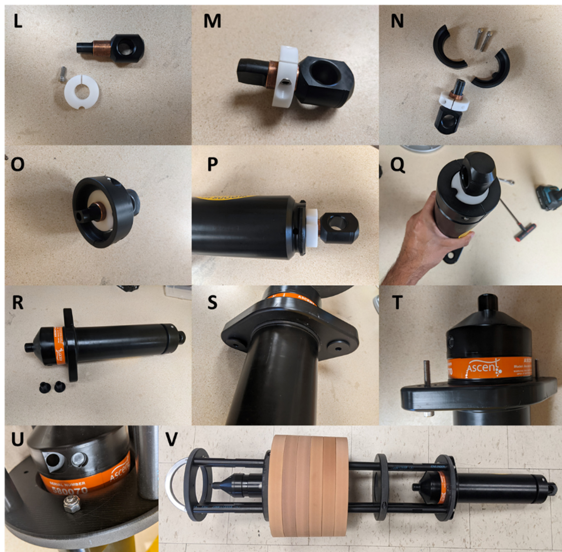
Fig. 3. L-Q) Assembly steps of the anti-shock collar and ring. R-U) Steps to attached the acoustic release to the TOSSIT frame. V) Assembled TOSSIT mooring without anchor.
