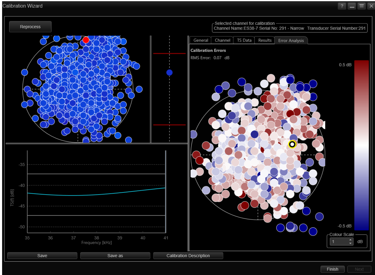
Figure 29. Screenshot of EK80 Calibration Wizard error analysis for the 38 kHz calibration at 1.024 ms in continuous wave (CW) mode.
