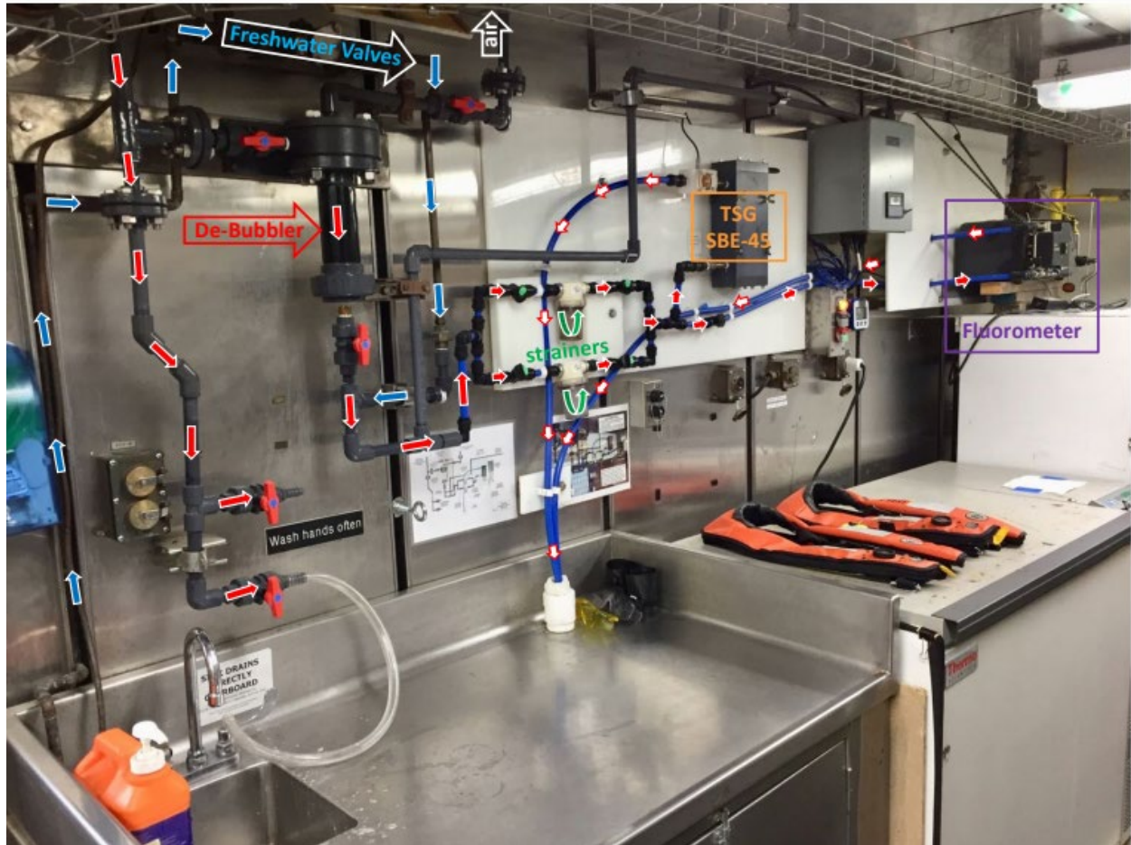
Figure 5. Flow diagram of Scientific Seawater System components in the wet lab, including the TSG. Photo: SST Wilkins.
